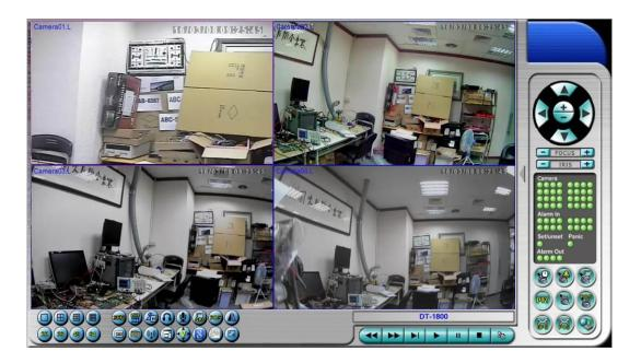
The video images can be displayed in several types of split-window screens, including 1/4/9/16/25/36/49/64 for DVRs. And the focus window is surrounded by a frame border. In addition to the video windows, there are different icons on the lower corner and the right corner of the screen for status display and control. (The ".L" following the camera title stands for Live display, ".P" for Playback, and the camera title with white background has detected motion.)
