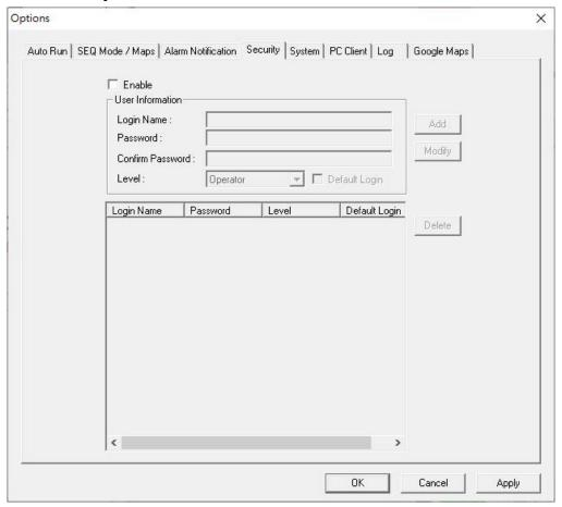
The system allows virtually unlimited number of user accounts. There are two password levels in the system, including **Administrator** (highest) and **Operator** (lowest). The Operator can only operate in Running Mode, but cannot change the configurations. The Administrator can do everything in Editing Mode and Running Mode.
