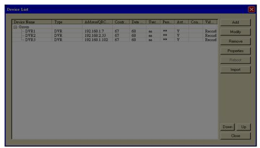
Please note that the devices for all the examples are already built in the device list. If the PC is connected to some devices, the user may modify the (IP address, Port Number,) Username & Password, and then run the HEM maps (Please refer to Chapter 4 – HEM Running Mode) in the Examples to get a better understanding of CMS Server.
