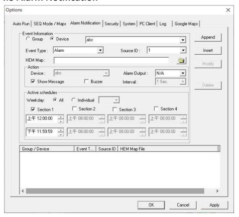
**Alarm Notification** is used to define how CMS Server responds to the alarms reported from the front-end devices in Running Mode.
