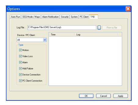
Please select the **Log File**, **Device**, and **Type of Log**, and then click on "**Apply**" to display the corresponding **Log List** in the dialog.
