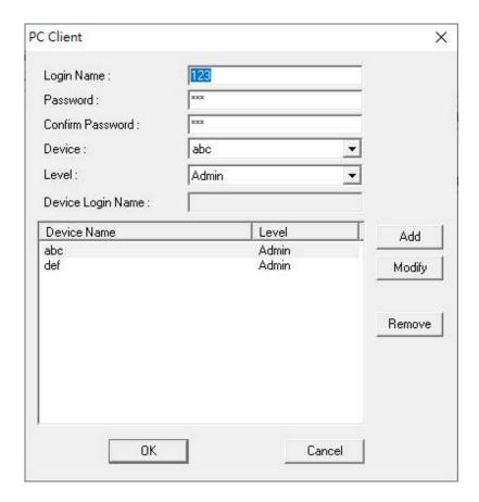
Please enter the **Login Name** and **Password** for this PC Client, and then add the **devices** to be monitored and controlled by the PC Client and its access **level** for each device respectively. Please click on **OK** button to save the settings, or **Cancel** button to exit without saving.
