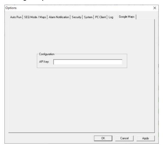
The API key paid for Google Maps can be set here. If users do not have API key, the query times for address and the load times of map for all users will be limited to 900 times per day totally for the built-in vendor provided API key after Jun. 11, 2018.
